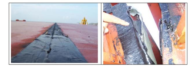
Seemingly, it looks like an additional precaution to enhance weathertightness. However, there are negative aspects to using hatch cover sealing tapes which include:-
